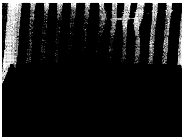
Figure 2 SEM of 0.14 \mu\text{m} L/S pattern of ArF photoresist
